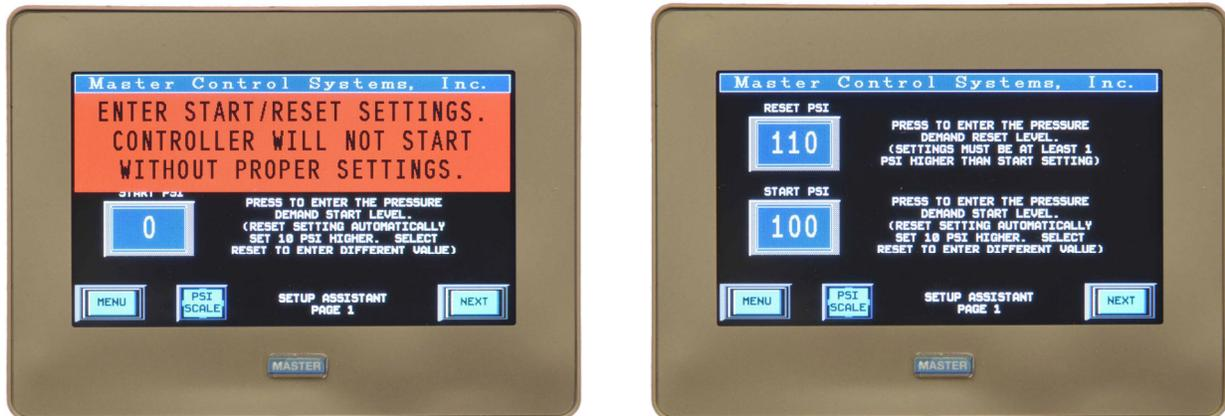
If you need to adjust your Reset Pressure Setting, simply push the RESET PSI (BAR) button, and set it accordingly.
