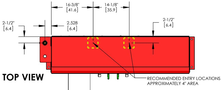
RECOMMENDED CONDUIT ENTRY AREA AT BOTTOM OF CONTROLLER. AREA IS APPROX 8-1/4" x 17-1/4"
