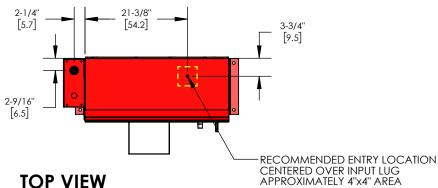
3-3/8" 8.6 RECOMMENDED CONDUIT ENTRY AREA AT BOTTOM OF CONTROLLER. AREA IS APPROX 7" x 23-1/4" 9-3/4" [24.8] 2-1/2" Ø9/16" [6.4] [1.4] 32" MOUNTING HOLES 81.3
