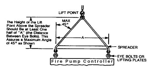
Figure 2-1 LIFTING WITH EYE BOLTS OR LIFTING PLATES
